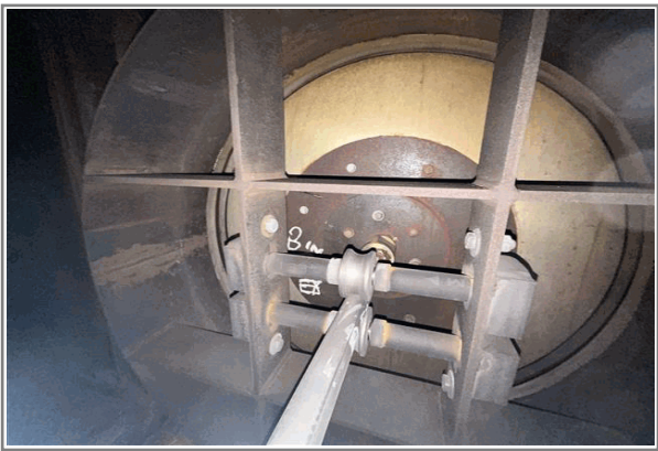
Poppet Valve & Roller Bearings (Chamber 1)
